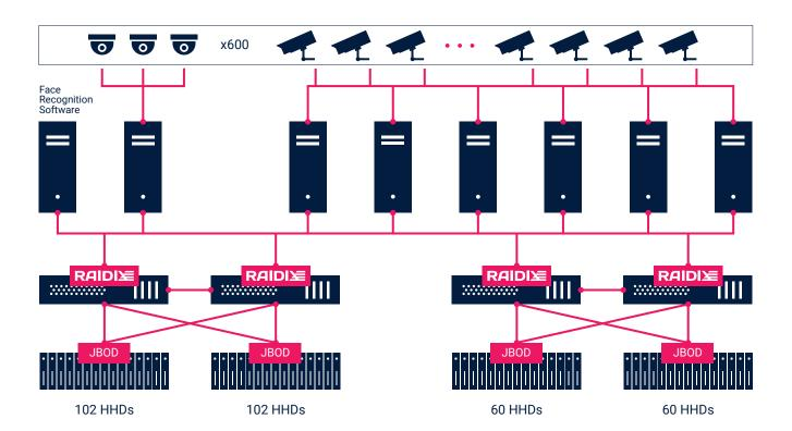
Each of the two RAIDIX-based storage systems provides up to 17GB/s bandwidth for read and write operations. This is almost **three times more** than the total peak load from 8 video servers (about 5GB/s).
