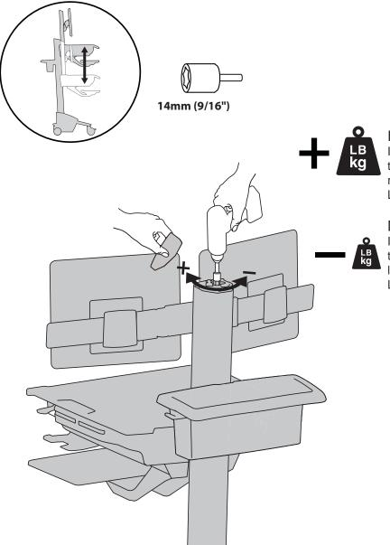
Increase Lift Strength If the mounted weight is too heavy or this product does not stay up when raised, then you'll need to increase Lift Strength:
