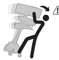
Warning: Not intended for use with SV40, 41, and 42/44 LiFe carts. These configurations create a tipping hazard when the height adjustment assembly and monitor are at maximum height. Failure to heed this warning may result in serious personal injury or property damage!
