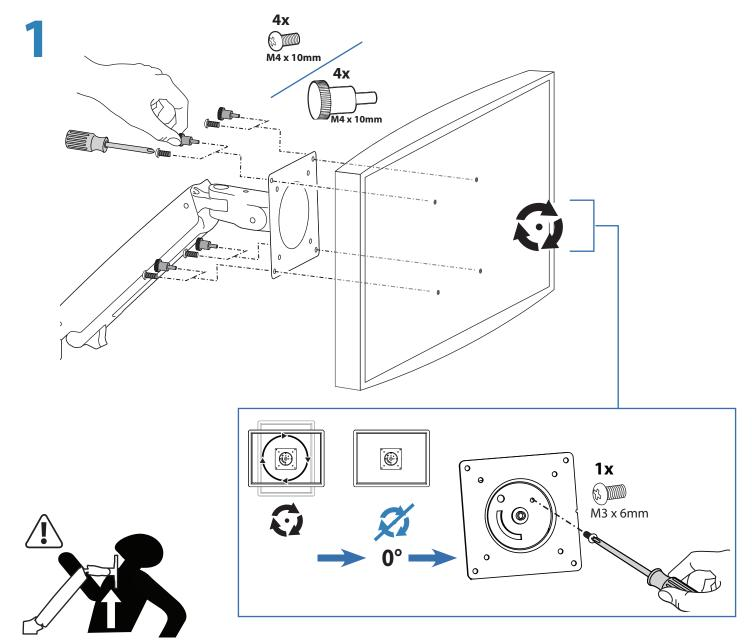
WARNING! Stored Energy Hazard: The Riser mechanism is under tension and will move up rapidly, on its own, as soon as attached equipment is removed. For this reason, DO NOT remove equipment unless the Riser has been moved to the highest position! Failure to follow this instruction may result in serious personal injury and/or equipment damage!
