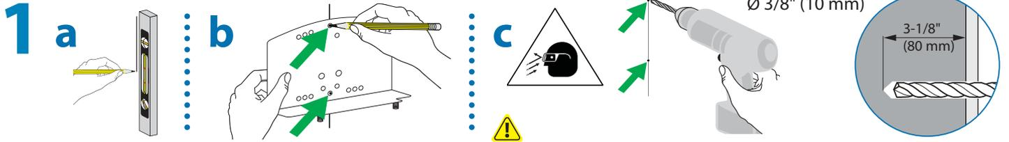
**WARNING:** Mounting holes must be at least 3-1/8" (80mm) deep and must be located within solid concrete, not mortar or covering material. If you drill into an area of concrete that is not solid, reposition mounting holes until both anchors can be fully inserted into solid concrete!
