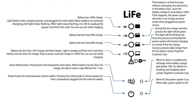
If other lights are flashing red/green it could indicate a power system fault. If this occurs contact Ergotron Customer Care.
