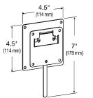
Front View (FX30 showing 75 x 75 mm monitor bracket attached to wall bracket)
