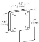
Front View (FX30 showing monitor bracket with 100 x 100 mm monitor adapter plate attached to wall bracket)
