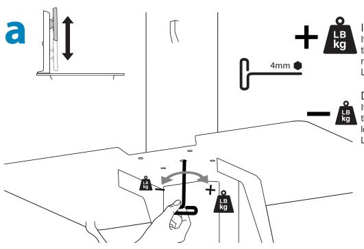
Increase Lift Strength If the mounted weight is too heavy or this product does not stay up when raised, then you'll need to increase Lift Strength:
